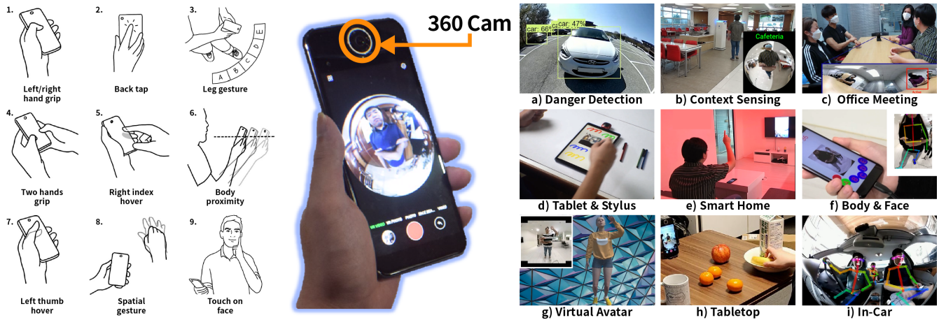
Figure 1: A mobile device with an omni-directional camera can capture a wide range of information about the user, including user’s hand, body, and the surroundings. This allows various sensing techniques, which enable novel applications for mobile interaction, including danger detection while on the move, body pose for virtual avatar, spatial gestures for gaming, and more.
