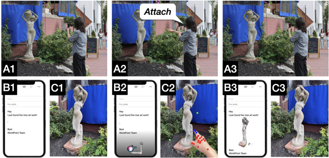
Fig. 9. In this example sequence, a user is composing an email on their smartphone (A1 & B1). Without exiting the email client, the user points with their finger at a statue they have found (A2). This acts as a "wake gesture" and the phone begins to track what the user is pointing to via its rear-facing camera (C2) and LiDAR, offering a small onscreen preview (B2). Simultaneously, the phone begins to listen for spoken commands. The user says "attach" (A2), which causes the statue to be added to the email (B3). The user then drops their hand (A3) and continues on their way. A1-3: External reference photos; B1-3: Interface screenshots; C1-3: Views from a phone camera, unseen by the user. See also Figure 1 for different steps of the data pipeline.
